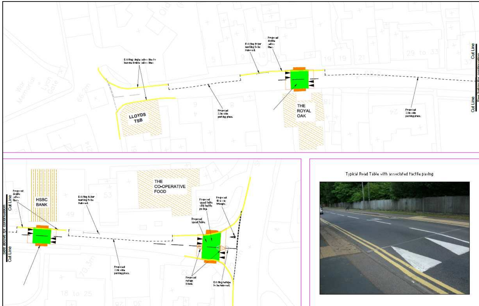
Option 3 – High Street to remain two-way with provision of passing places and pedestrian crossing points
